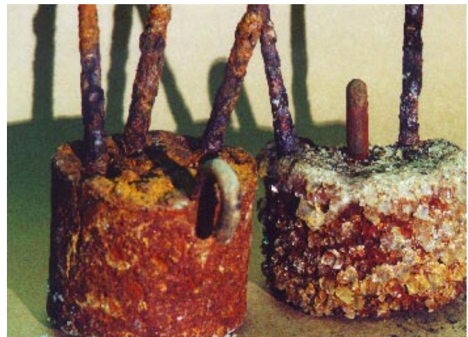
Figure 3. Photograph of IPANEX concrete [left] and the control concrete [right] rotated 180°.
