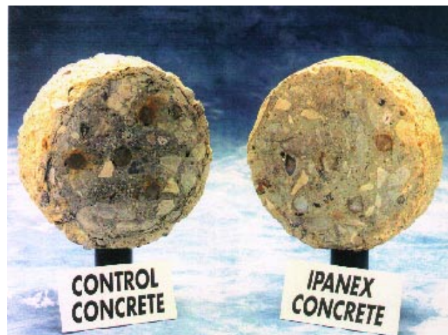
Figure 1. Control and IPANEX concrete cylinders exposed to oil well brines.
