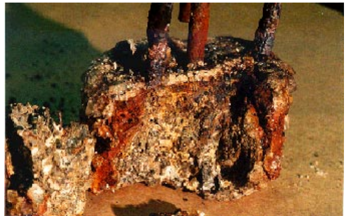
Figure 6. Photograph of the control concrete after alternate exposure to 7 years 3 months in brine and 1 year 3 months in air.
